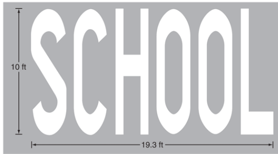
Figure 7C-1. Two-Lane Pavement Marking of "SCHOOL"
